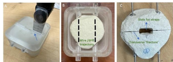
Fig. 2 A. Transverse slots (arrow) in jig to guide saw cut.
