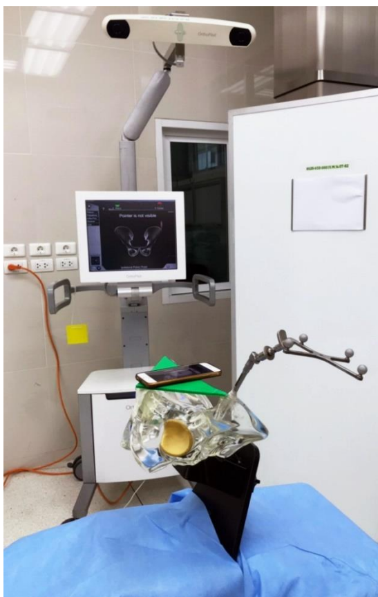
Fig.1 The pelvic model was positioned and fixed firmly in the supine position on a flat table. The Orthopilot imageless navigation system was located on the opposite side.
